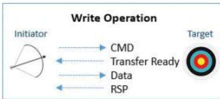
Figure 2 - FCP Write Operation
