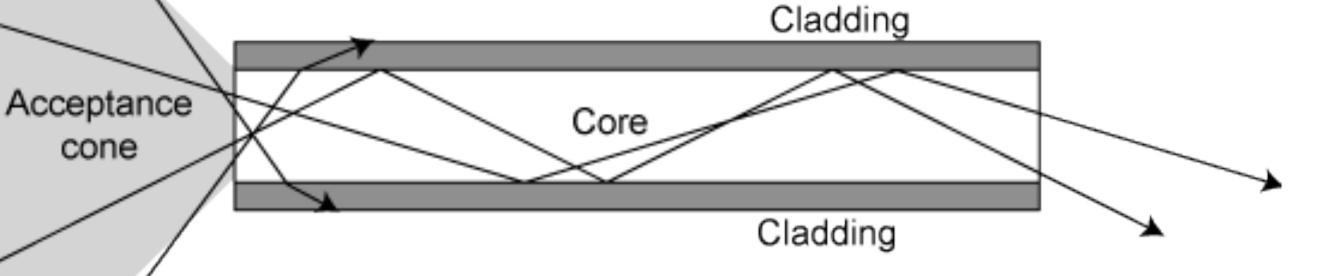
When the light tries to pass from the core to the cladding, and the angle is correct, it is reflected back into the core.
